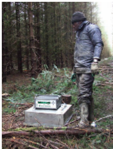
Figure 2: CO 2 and trace gas measurements being measured using a photoacoustic analyser on brash lines after the second thinning at Dooary (20-year-old stand).
